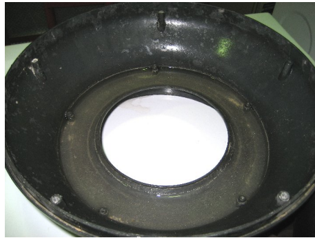
Figure 3 – Sample 1, water pooling inside housing and dripping down inside of enclosure
