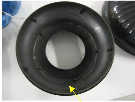
Figure 5 – Sample 2, The Engineer noted water pooling inside housing and dripping down inside of
